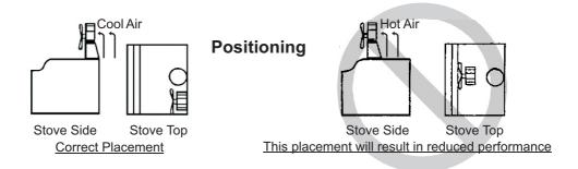
NOTE: Overheating will reduce the Ecofan's effectiveness and may damage the power generator and void the warranty. Remove the Ecofan from the stove if temperatures exceed 340°C (650°F)
